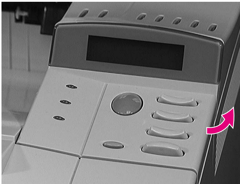
Figure 41. Removing the control panel overlay
